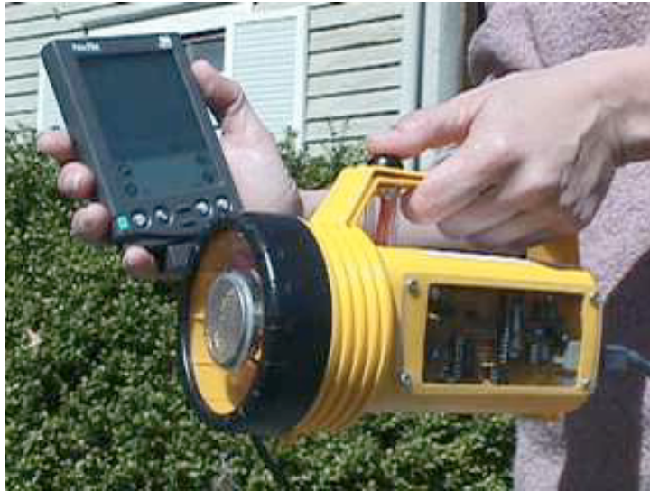
Figure 3. The smart motion detector interfaced to a Palm handheld computer. The ultrasonic transducer can be seen mounted in the face of the flashlight case. The PIC microprocessor and other electronics can be seen through the window of the case. The Palm display on the right shows time-graphs of the position (lower trace) and velocity (upper).
